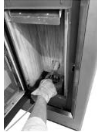
Fig. 36 - Cleaning with a brush
